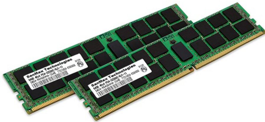
DIMM (Dual Inline Memory Module)
